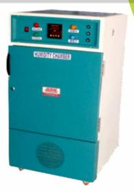
Machine is used to conditioning of the samples at specified temperature as well as specified humidity. Humidity range 50% to 95%. Temperature range 20°c to 45°c Suitable standards are IS, ASTM or other equivalent standards. Machine suitable for Pipes, woven fabrics, woods, flexible pouch for food grade.
